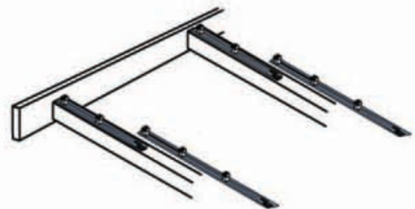
图3 Figure 3 安装好第一排固定座后，顺次安装 下面的固定座和面板 Fix the first row of clips. Fix the next (and subsequent) clips and sheets
